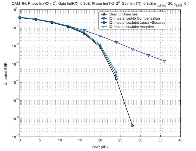
(a) AWGN flat channel (*non-fading*).
