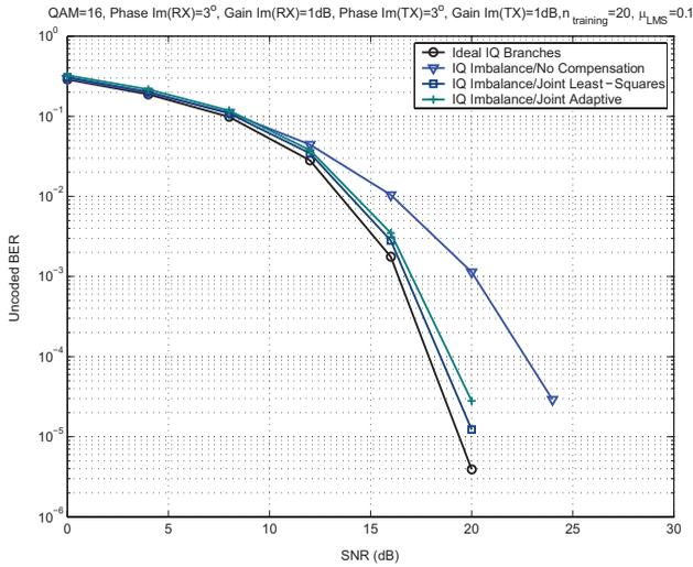
(a) AWGN flat channel (*non-fading*).
