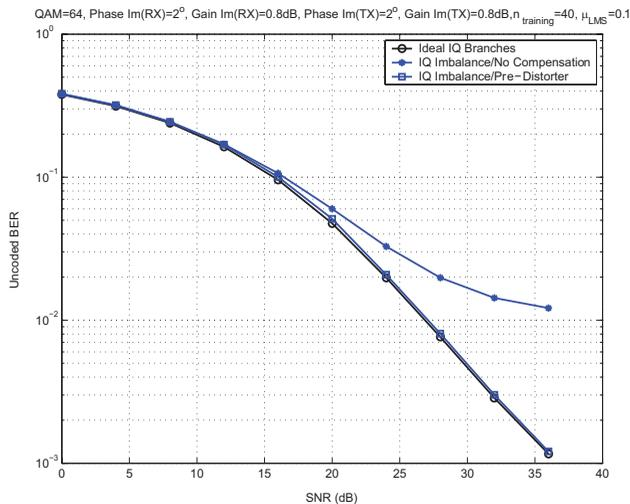
Fig. 6. BER vs. SNR simulated for the following configuration: 4-tap complex Gaussian fading channel, 64QAM constellation, training length of 40 OFDM symbols, transmitter phase imbalance of  $\theta_t = 2^\circ$ , transmitter amplitude imbalance of  $\alpha_t=0.8\text{dB}$ , receiver phase imbalance of  $\theta_r = 2^\circ$ , and receiver amplitude imbalance of  $\alpha_r=0.8\text{dB}$ . ‘IQ Imbalance/Pre-Distorter’ refers to the compensation scheme in defined by (40) and (43).
