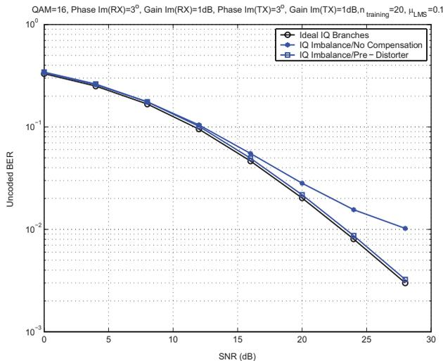
Fig. 5. BER vs. SNR simulated for the following configuration: 4-tap complex Gaussian fading channel, 16QAM constellation, training length of 20 OFDM symbols, transmitter phase imbalance of  $\theta_t = 3^\circ$ , transmitter amplitude imbalance of  $\alpha_t=1\text{dB}$ , receiver phase imbalance of  $\theta_r = 3^\circ$ , and receiver amplitude imbalance of  $\alpha_r=1\text{dB}$ . ‘IQ Imbalance/Pre-Distorter’ refers to the compensation scheme in defined by (40) and (43).
