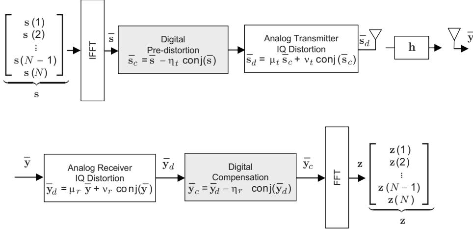
Fig. 2. An OFDM system with post-IFFT transmit and pre-FFT receive compensation for IQ imbalances. The gray blocks depict the compensation operations. Note that the addition and removal of the cyclic prefix are not shown in the figure for ease of notations.
