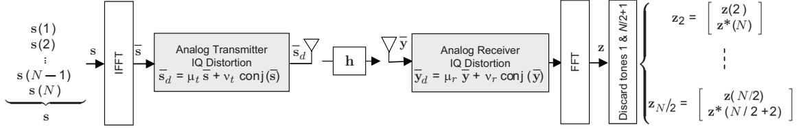
Fig. 1. An OFDM system with both transmit and receive IQ imbalances and the notation used in the derivations. Note that the addition and removal of the cyclic prefix are not shown in this figure for ease of notations.
