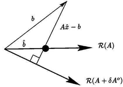
Fig. 3. Orthogonality condition for BDU estimation.
