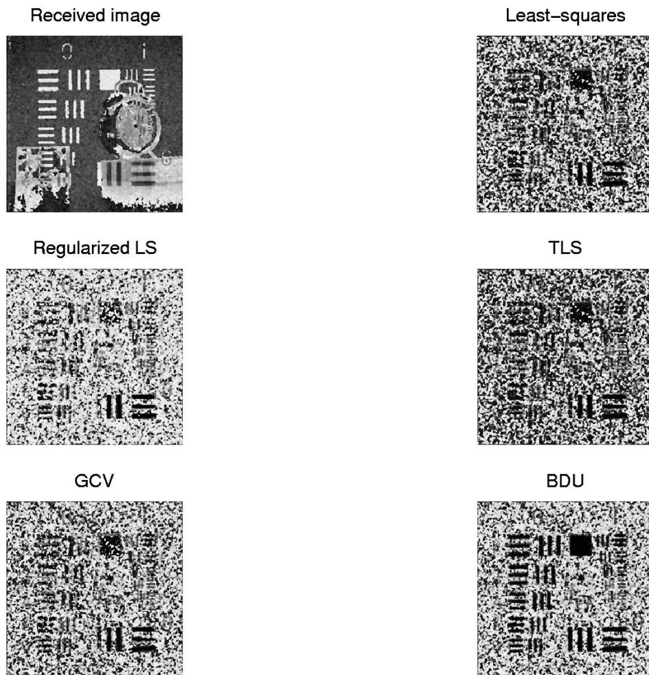
Fig. 7. Received image at the left-most antenna in addition to the chart images that are recovered by the LS, regularized LS, TLS, GCV, and BDU methods followed by  $3 \times 3$  median filtering. The chart image is the one that is transmitted over the nominal channel  $A_2$  with relative uncertainty bound 25%. In this case, the BDU solution recovers more details.
