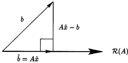
Fig. 2. Orthogonality principle:  $A\hat{x} - b \perp \mathcal{R}(A)$ .
