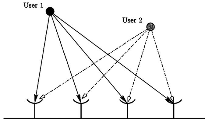
Fig. 1. Spatial processing with multiple users and antennas.
