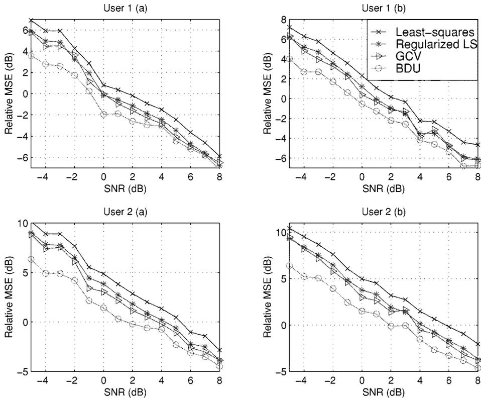
Fig. 4. MSE curves for both users 1 and 2 in a 4PAM modulation scenario with perturbation bounds  $\eta_1 \approx 15\%$ ,  $\eta_2 \approx 25\%$ . The plots (a) correspond to random perturbations within the permissible bounds. The plots (b) correspond to maximal perturbations (on the boundary). Each point in the plots was obtained by averaging over 300 transmissions.
