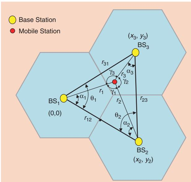
[FIG5] A schematic of a cellular network topology with three BSs.
