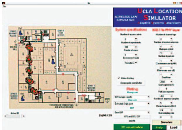
**[FIG9]** An illustration of the UCLA WLAN Location Simulator interface. The estimated location of a mobile user using different algorithms would be plotted for different realizations. Moreover, the estimated accuracy of the different methods would be shown by circles surrounding the mobile location.
