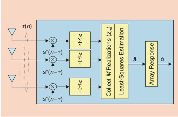
**[FIG8]** AOA estimation using an antenna array over a single path fading channel.
