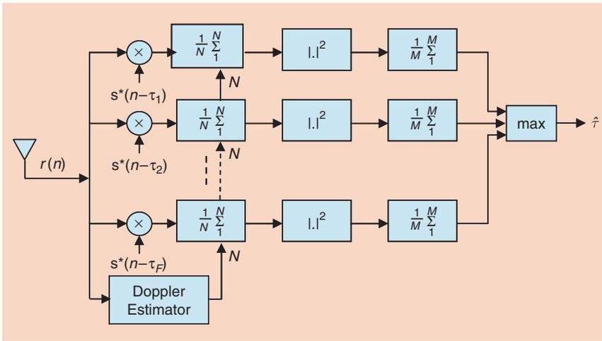
**[FIG6]** A scheme for TOA estimation over fading channels.
