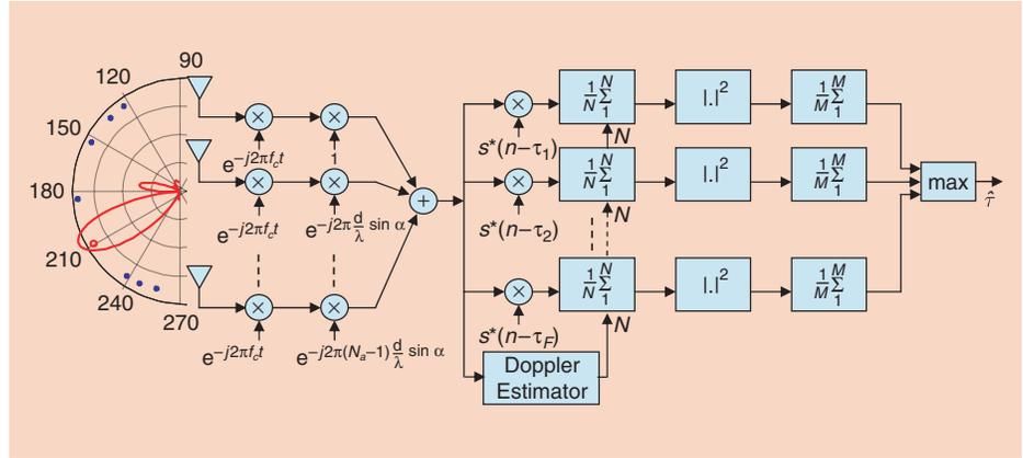
**[FIG7]** TOA estimation over fading channels using an antenna array.
