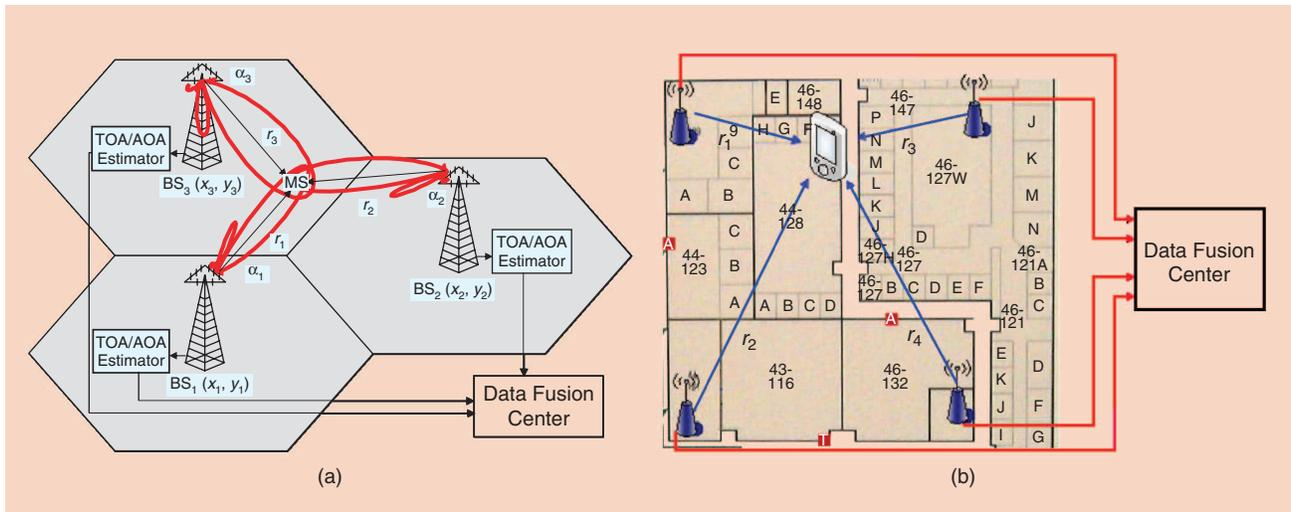
[FIG2] Network-based wireless location finding. (a) Outdoor environment using a cellular network. (b) Indoor environment using a WLAN.
