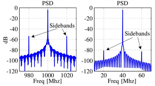
Fig. 2. The left figure shows the PSD of the distorted PLL clock and the right figure shows the PSD of the sampled sinusoidal tone.
