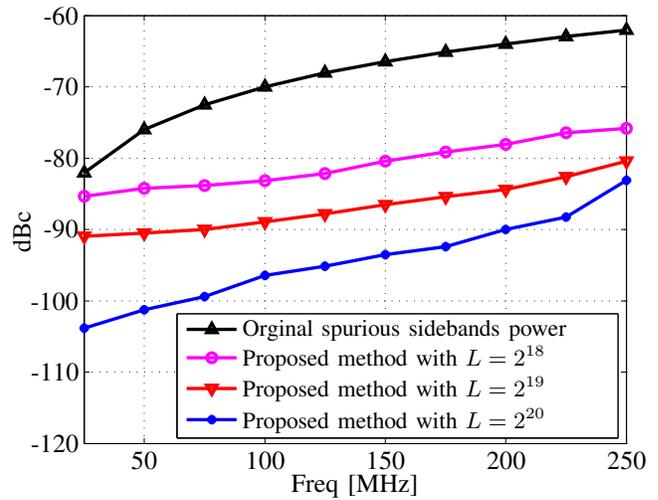
Fig. 6. A sinusoidal input is sampled using the distorted PLL clock. The plot shows the relative power of the spurious sidebands (in the sampled data) to the power of the input tone before and after compensation. The value  $L$  represents the length of the sequence that is used in the parameter estimation algorithm.
