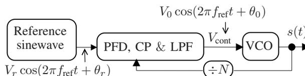
Fig. 1. Block diagram of a PLL
