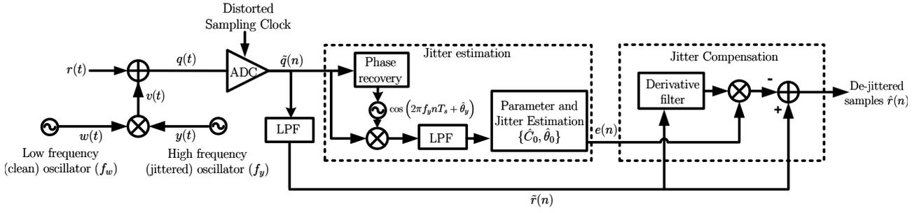
Fig. 3. Proposed architecture for sideband reduction on A/D converters due to spurious PLL tones.
