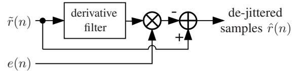
Fig. 4. Block diagram of the sideband suppression scheme.
