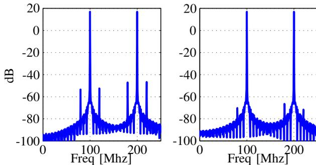
Fig. 5. The left figure shows the PSD of the sampled data. The right figure shows the PSD of the compensated signals using the proposed architecture.
