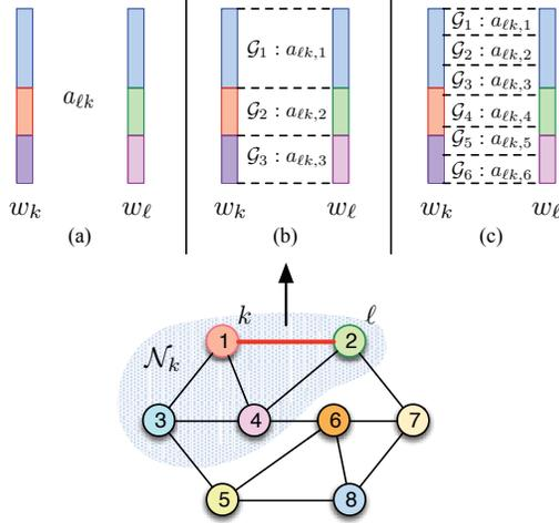
**Fig. 1.** Network model for group diffusion LMS. (a) Weight vector structures for nodes  $k$  and  $\ell$ , where three sections coded by colors exhibit different levels of similarity; (b) optimal groups; (c) groups with uniform sizes.
