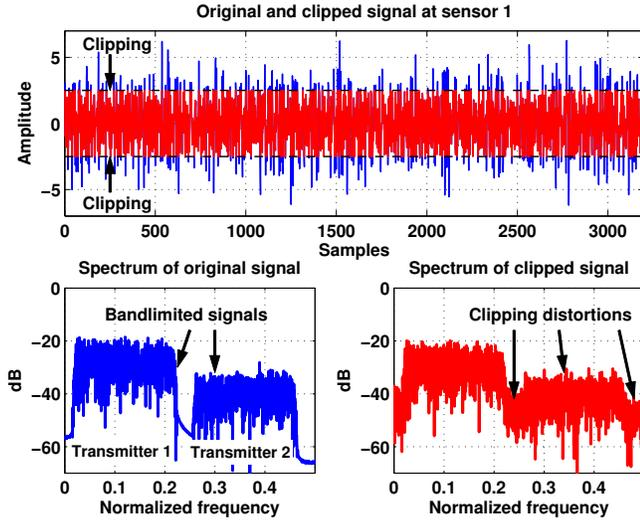
Fig. 2. The plots show both the time-domain and frequency-domain of the original and clipped signals at sensor 1. Details of the simulation parameters are in Section 2.3. The clipping level CL is  $\pm 3.5$ .
