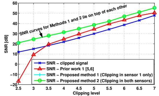
**Fig. 3.** The plot shows the SNR of the clipped signal and the recovered signal using Prior work 1 [5,6], Methods 1 and 2. (Method 1 is used when only sensor 1's data has clipping distortion, and Method 2 is used when both sensors' data have clipping distortions.)
