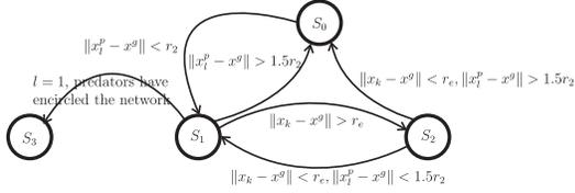
**Fig. 3.** State transition diagram of the motion model of predators.
