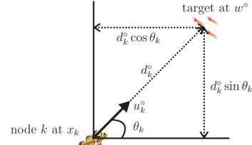
**Fig. 1.** Distance and direction of the target  $w^\circ$  from node  $k$  at location  $x_k$ . The unit direction vector  $u_k^\circ$  points towards  $w^\circ$ .
