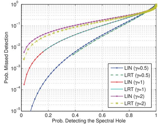
**Fig. 2.**  $(1 - P_d)$  versus  $(1 - P_f)$ , with  $N = 2$  and various  $\gamma$  values.
