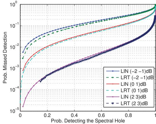
**Fig. 1.**  $(1 - P_d)$  versus  $(1 - P_f)$ , with  $N = 2$  and  $\gamma = 2$  at various SNR levels. The SNR levels of the two CRs are given in the parentheses.
