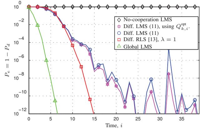
Fig. 3. Probability of error ( $P_e = 1 - P_d$ ) for  $P_f = 10^{-9}$ .
