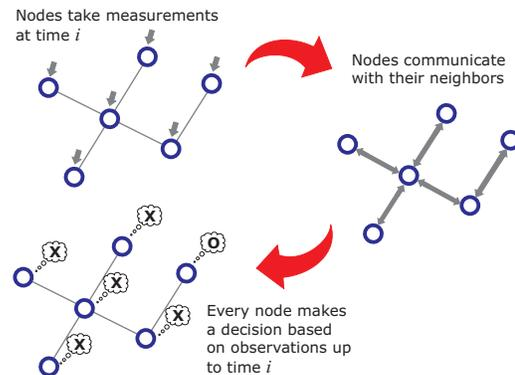
Fig. 1. Distributed detection scheme.
