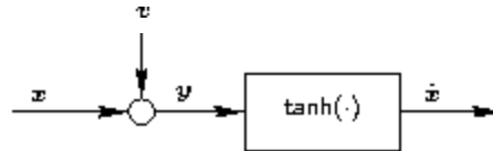
Figure 1.3. Optimal estimation of a BPSK signal embedded in unit-variance additive Gaussian noise.
