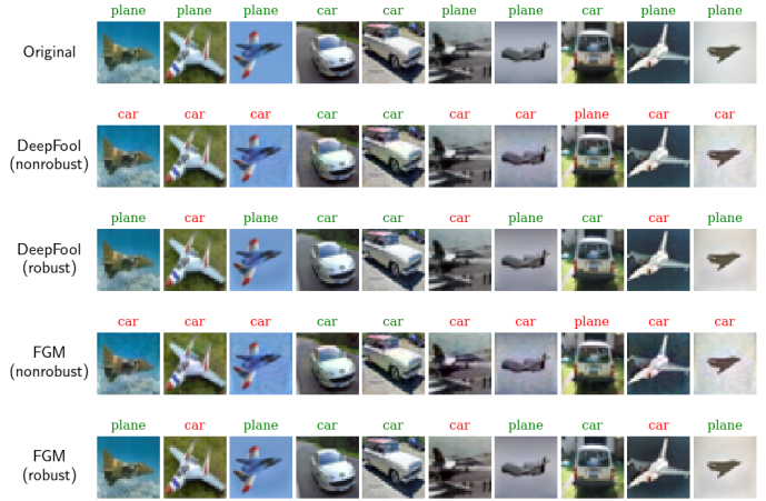
Fig. 4. Visualization of the original and adversarial samples. The first row consists of 10 random original samples with the titles representing their true classes. The second row shows the adversarial examples generated by DeepFool and applied to the standard (nonrobust) algorithm. The third row shows the results obtained by the adversarial (robust) algorithm. The titles are the predictions by the corresponding models. The same construction is repeated in the last two rows using FGM. If the prediction of an image is wrong, the title is shown in red color. It is seen that the adversarial algorithm fails less frequently.
